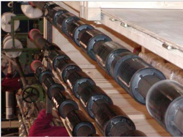
Figure 4: Expandable zonal isolation profiler tool with feed-through capability for control liners.
